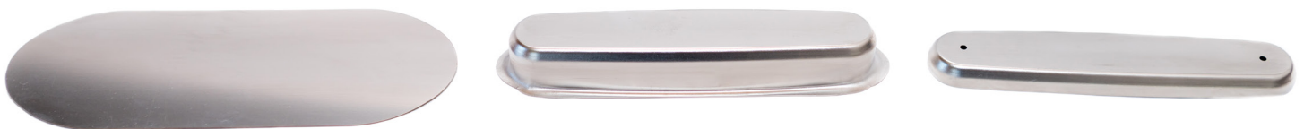
(Example of a hydroformed part from flat blank to in-process part to final hydroformed part with laser cut details.)
